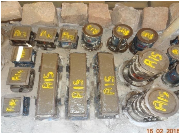
Fig 1: Moulds filled with concrete
