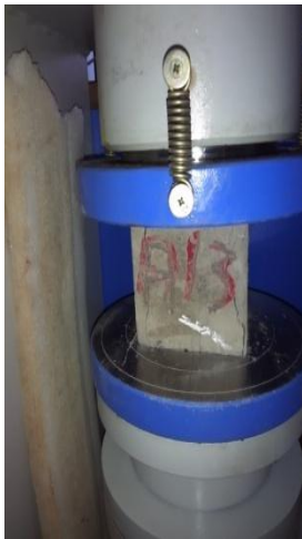
Fig 2: Compressive Strength Test
