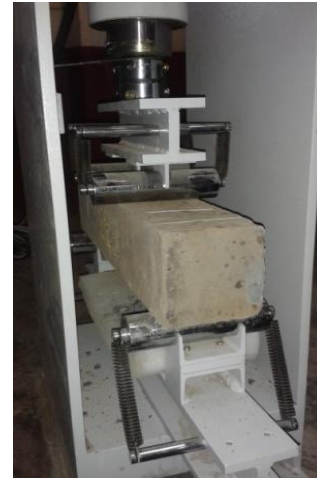
Fig 4: Flexural Strength Test
