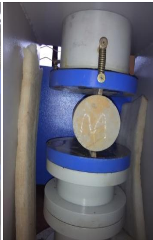
Fig 3: Split Tensile Strength Test
