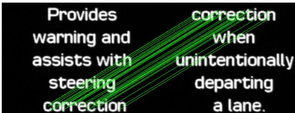
Fig. 3.10 Homogenous point matching using Brute force matcher for Vertical scrolling image
