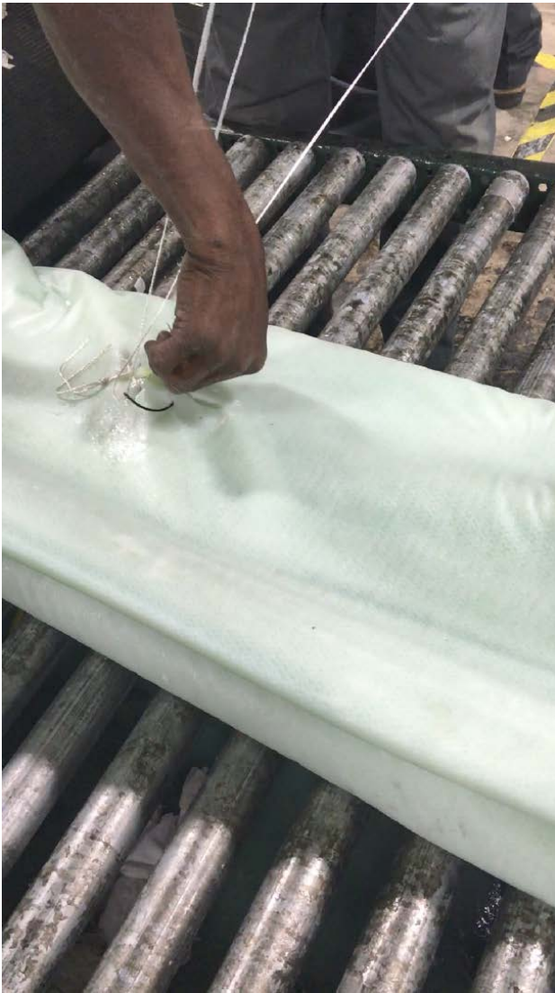
Figure A3. Employee repairing hole in completed liner at wet-out facility, December 2019. Photo by NIOSH.
