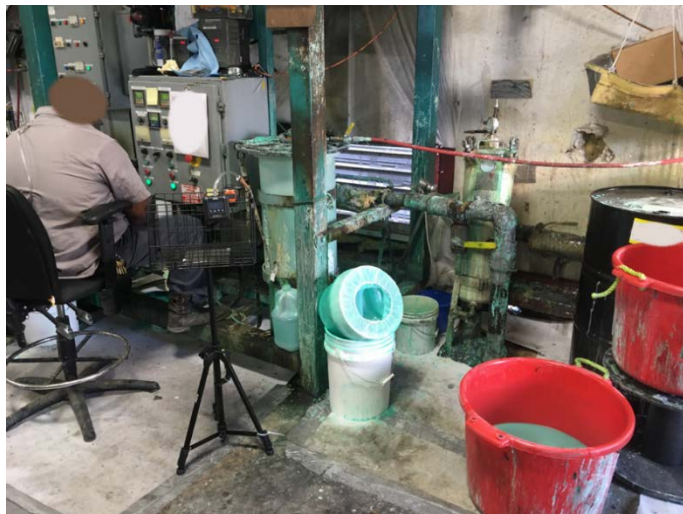
Figure A1. Employee sitting at controls of resin-pump static mixer station at wet-out facility. The red buckets contained styrene and catalyst. The white bucket with a filter on top was used to transfer styrene-catalyst mixture to the hopper of the resin-pump static mixer, located to the immediate right of the controls, December 2019. Photo by NIOSH.
