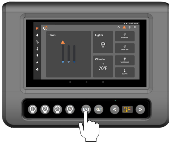
Figure 36: Press EXT to wake the display
