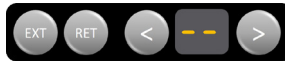
Figure 5: Node cannot connect to device. Clear memory to connect to a new device.
