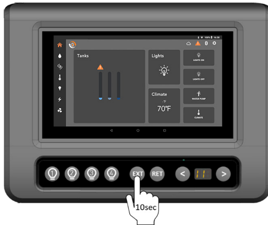
Figure 7: Navigate to 'PA' and press and hold EXT for 10 seconds to clear the Node memory
